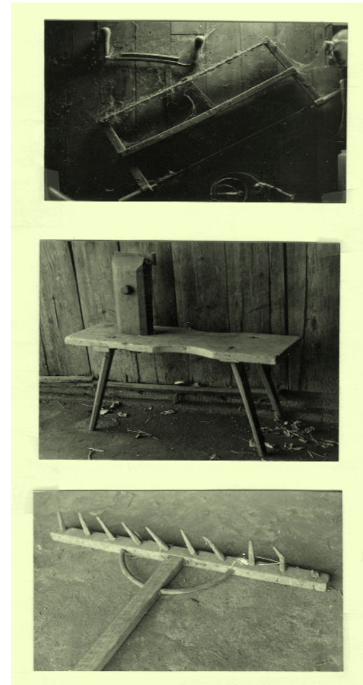
Figure 33 Early handmade tools: a bucksaw, a harness repair vice and a garden rake
