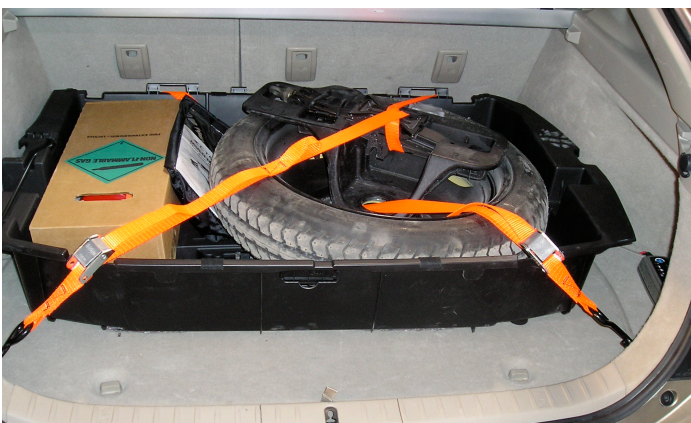
Quick-release tie-down straps used to secure spare-tire and jack equipment, as installed in unit #1989 (left) and unit #1982 (right)
