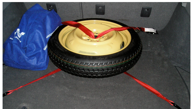
Quick-release tie-down straps used to secure spare-tire and jack equipment, as installed in unit #1989 (left) and unit #1982 (right)
