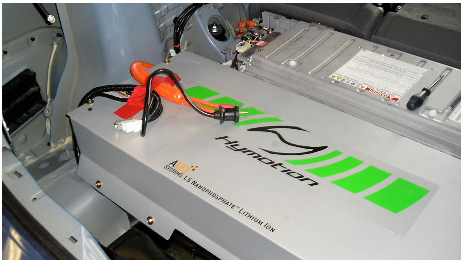
A123Systems Plug-in Conversion Module installed in the rear compartment area of Toyota Prius, behind nickel metal hydride stock hybrid battery
