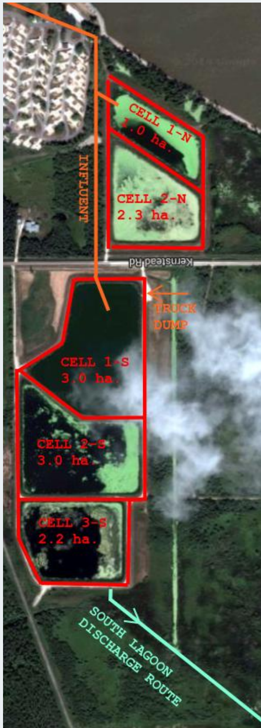
FIGURE 1: EXISTING LAGOON SYSTEM
