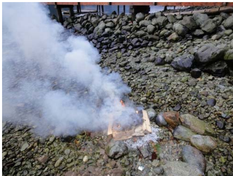
Photo 7. ASR Placed on small wood fire (time = 0 seconds)
