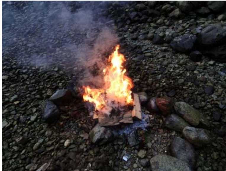
Photo 10. ASR fully involved in vigorous burn (t= 60 seconds)
