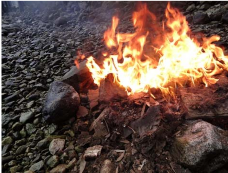
Photo 12. Flame front advancing 450 cm in 90 seconds
