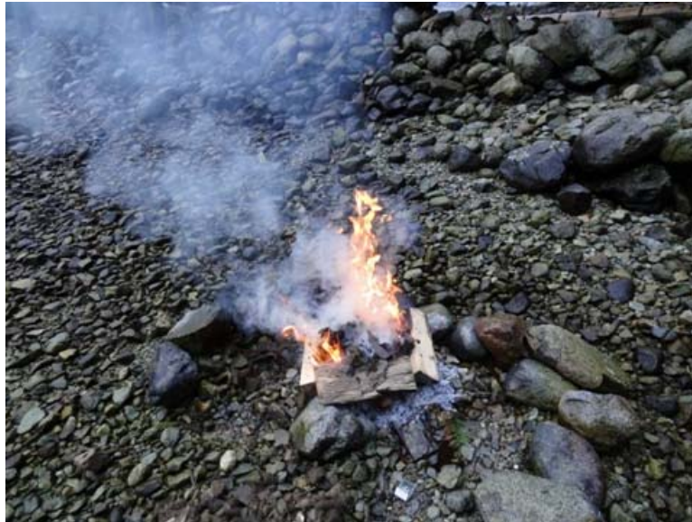
Photo 8. Combustion of ASR initiated (time = 15 seconds)
