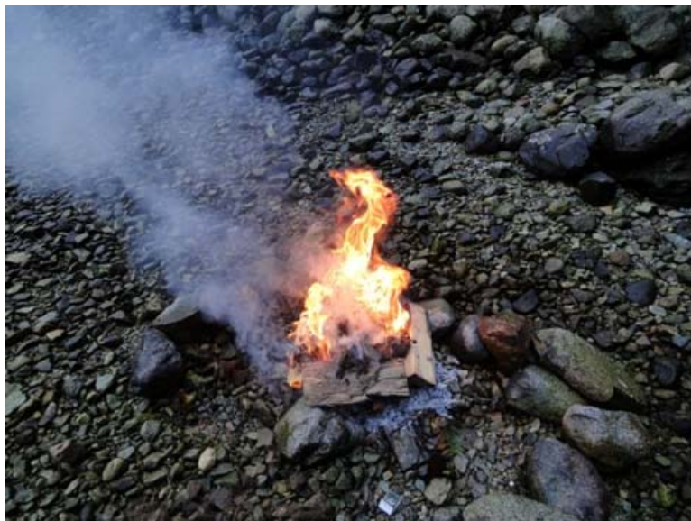
Photo 9. Fire in ASR Spreads (time = 30 seconds)
