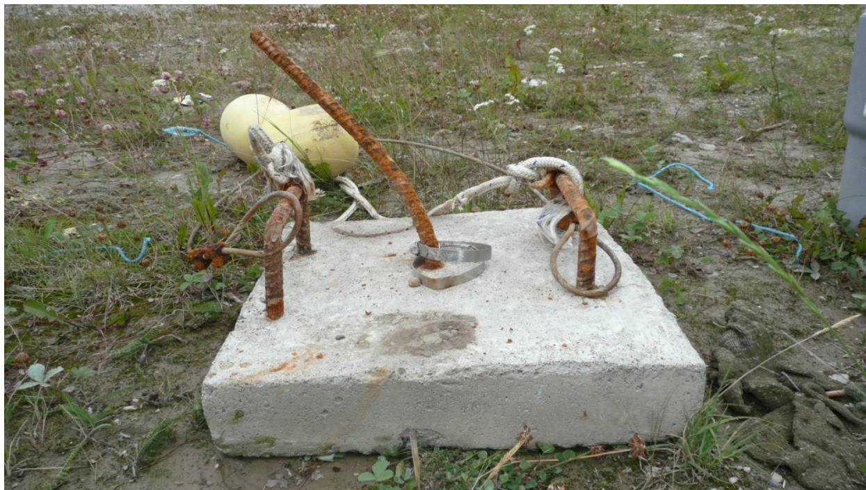
Photo 1. Receiver 4495 mooring damaged by ice over winter in Stephens Lake.
