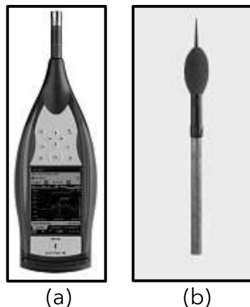
Figure 22: (a) Brüel and Kjær 2250-L Noise Meter; (b) Brüel and Kjær 4952 Microphone.
