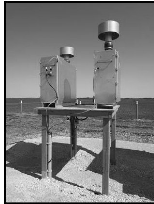
Figure 25: Ion counters mounted on table at north remote station.
