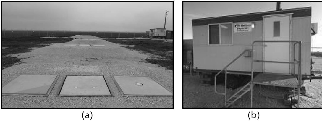
Figure 34: (a) Instrument gravel mound across ROW; (b) Main station trailer.
