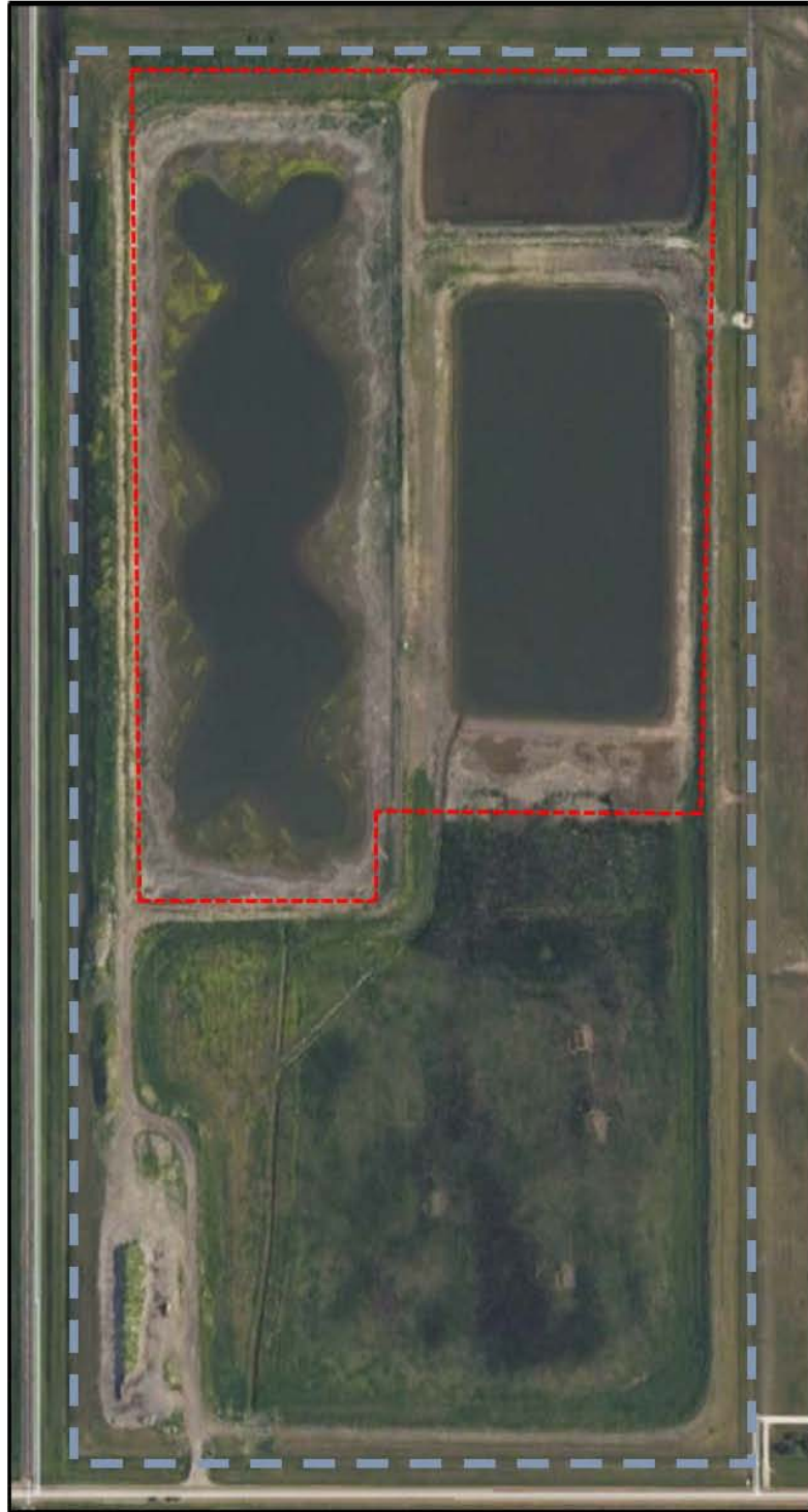
Figure 3. Recommended fencing location (red, dashed line) on the inside of the lagoon berms to limit access for those areas remaining under licence, should decommissioning of the dry cell be approved. Note that the fencing location shown is approximate and for discussion purposes only. The existing lagoon fencing (light-blue, dashed line) is also to be maintained. Image courtesy of Google Earth (Imagery date: June 2013).
