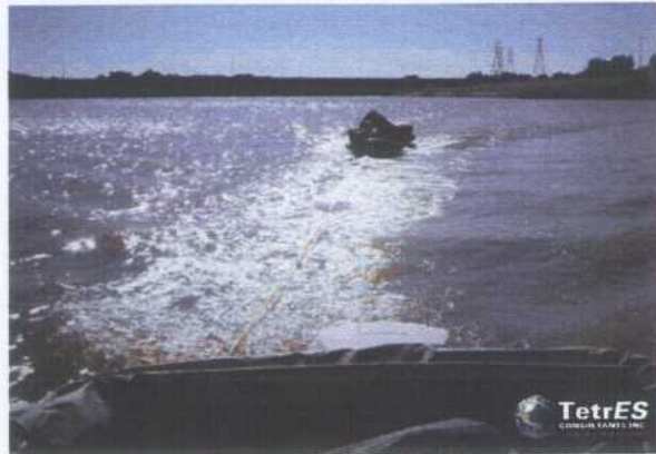
Figure 10: Moving the boom over longer distances was done by loading the boom in to a zodiac boat and towing it behind a speedboat.
