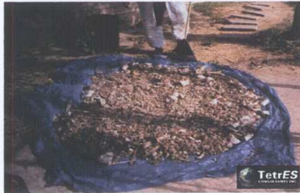
Figure 12: The first boom installation at the Alexander outfall yielded significant volumes of captured floatables. After one rainfall, the boom at this location captured almost 80 pounds of floatable debris.
