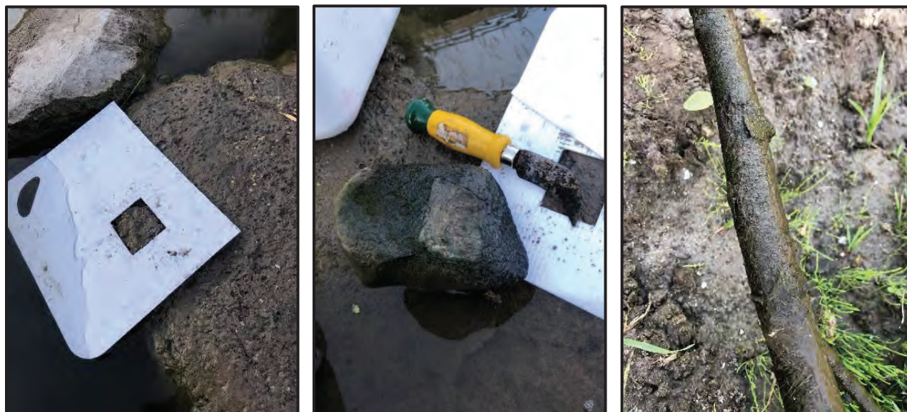
Figure 3-3 Periphyton Sampling using 5 cm x 5 cm Periphyton Templates, Rock after Periphyton Removed with Knife, and Woody Debris with Periphyton Growth at Site 2 (left to right)
