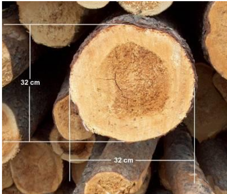
Figure 2 Measuring diameters: logs with regular sawn surfaces
