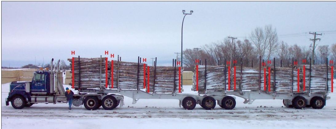
Figure 13 Height measurements taken on a loaded truck
