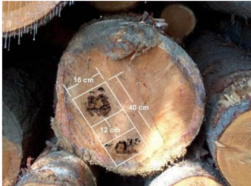
Figure 25 Two defects separated by 14 cm or less
