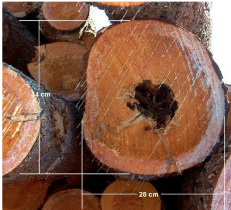
Figure 3 Measuring diameters: logs with irregular sawn surfaces
