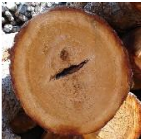
Figure 24 Heart check on the end surface of a log
