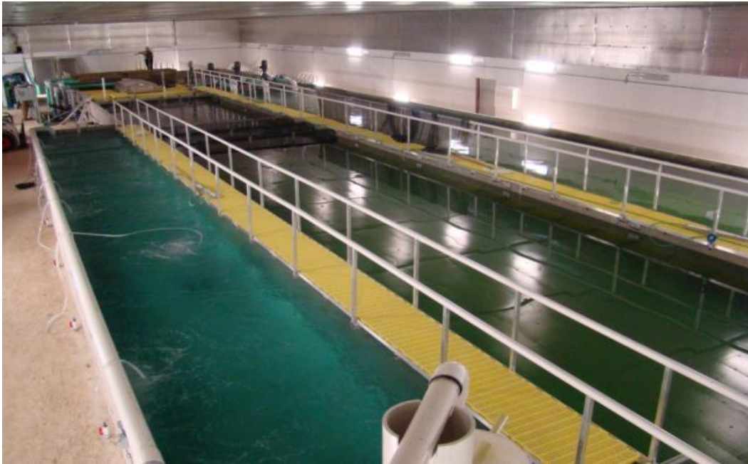
Figure 17: View of the production raceways and purge tank (on the left) with the incoming well water line in the foreground.
