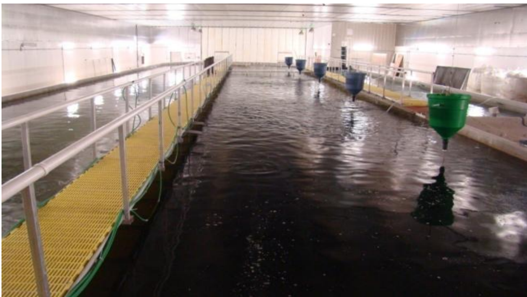
Figure 18: View of the production raceways and pendulum demand feeding system.
